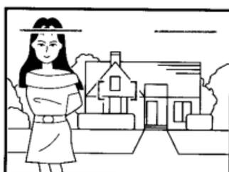
1. Center the AF frame over the subject. Press the shutter button lightly to focus the subject. The green indicator lamp lights up when the subject is in focus.
